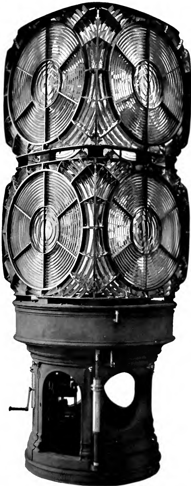
FIG. 54.—FASTNET LIGHTHOUSE—FIRST ORDER SINGLE-FLASHING BIFORM APPARATUS.
