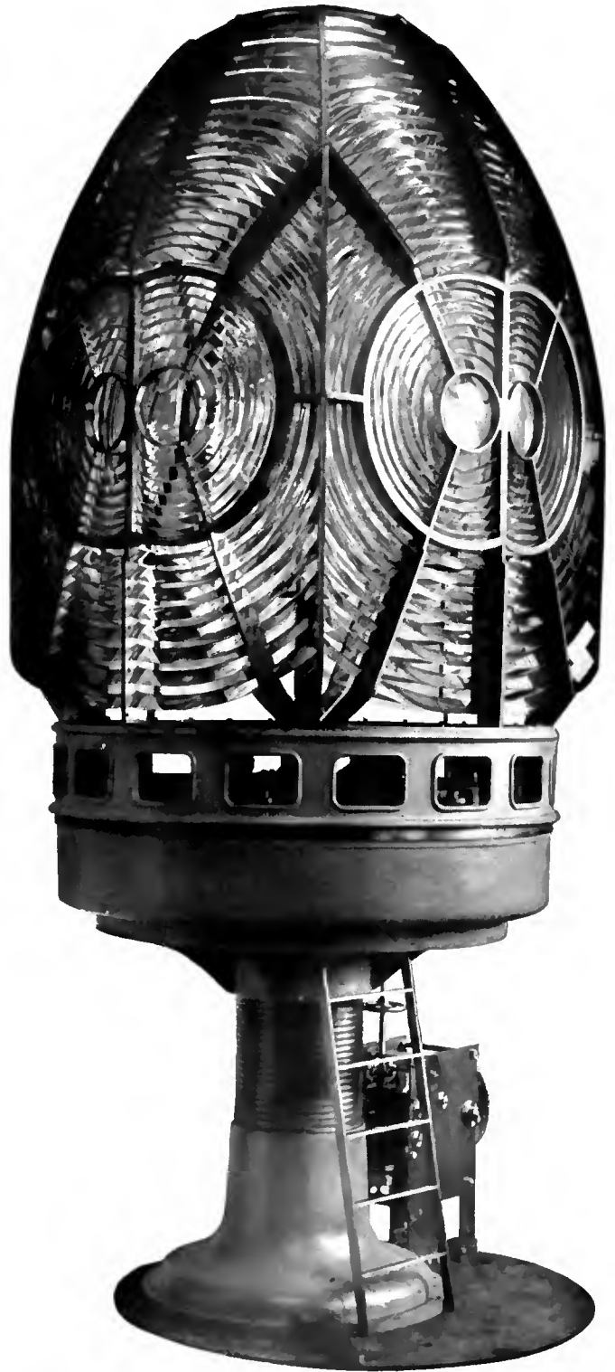
FIG. 55.—PACHENA POINT LIGHTHOUSE, B.C.—FIRST ORDER DOUBLE-FLASHING APPARATUS.
